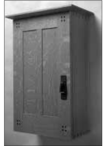
Wall Cabinet made by Chris during his Twelve-Week Intensive. Quarter-sawn white oak with ebony inlay. 24" tall, 14" wide, and 8" deep. April, 1998.
